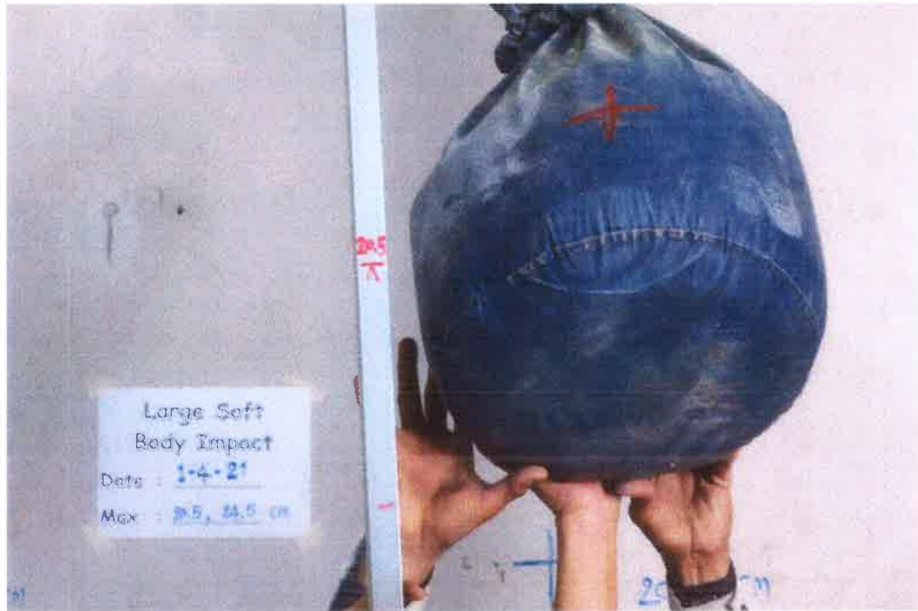
Figure 5 Drop height set up for testing of resistance to damage by impact from a large soft body impact
