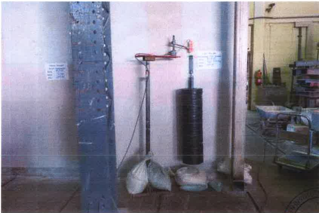
Figure 18 Release of shim plate at 2,942 N pull-down load
