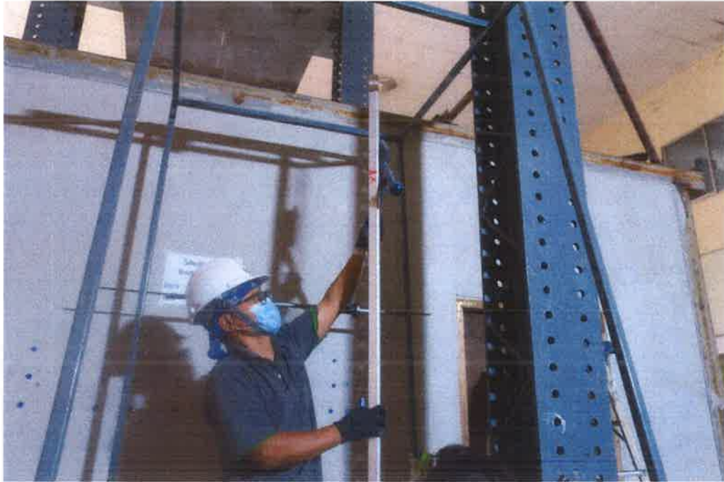
Figure 7 Drop height set up for testing of perforation by small hard body impact
