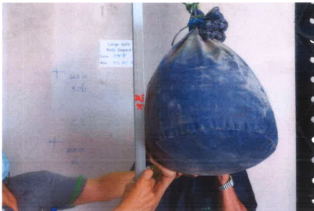
Figure 9 Drop height set up for testing of resistance to structural damage by multiple impacts from a large soft body
