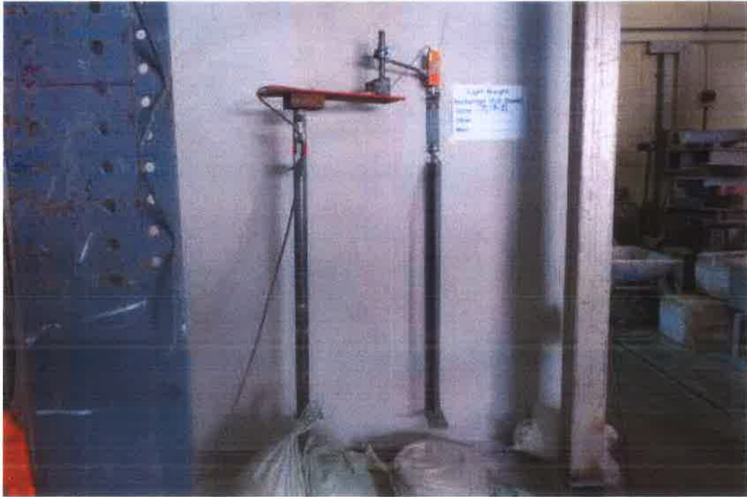
Figure 17 Lightweight anchorage pull-down test
