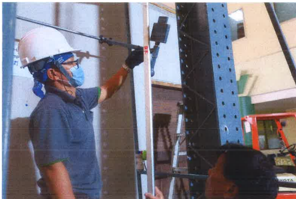
Figure 3 Drop height set up for testing of surface damage by small hard body impact
