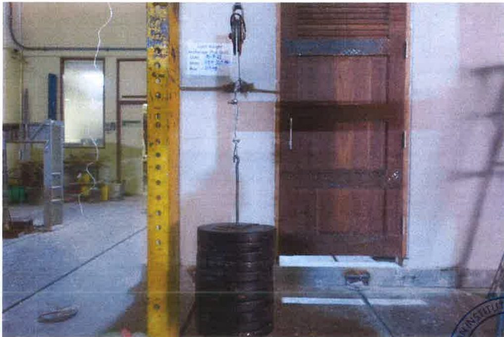
Figure 16 Release of shim plate at 1,079 N pull-out load
