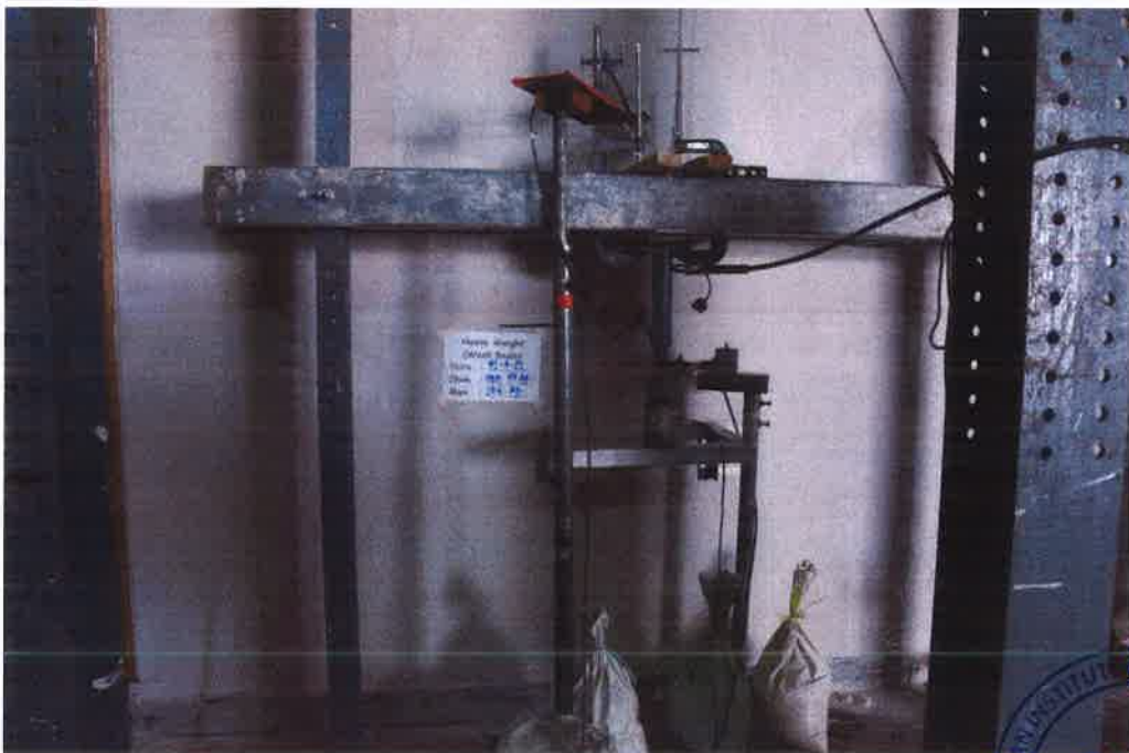
Figure 20 Release of shim plate at 539 N wash basin load
