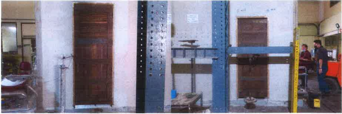
Figure 11 Equipment setup for testing of effects of door slamming
