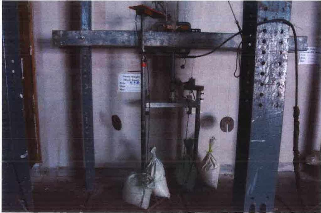
Figure 19 Heavyweight anchorage by eccentric downward loading (wash basin)
