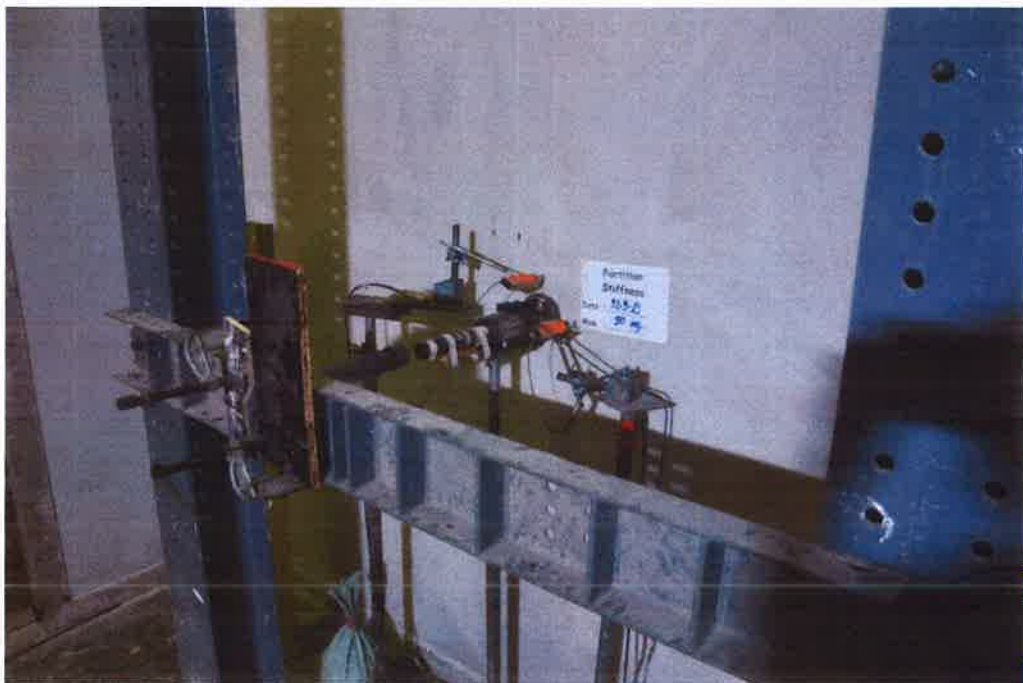
Figure 2 No damage after partition stiffness test
